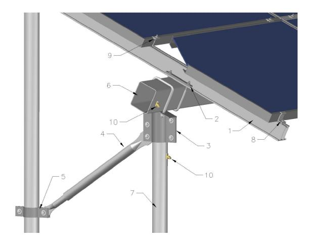
**1 - SF Rail:** Standard rail lengths are available for 4, 5 & 6 rows of panels in a landscape configuration. Custom lengths are available.
